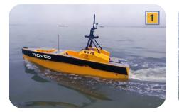
USV onboard for simultaneous data collection with instant upload to vessel, including MBES (R2sonic 2026-V MBES), SSS (EdgeTech 4205) and USBL (Sonardyne Mini-Ranger 2). Ability to run infill, nearshore and inshore surveys on its own, in parallel with mothership.
