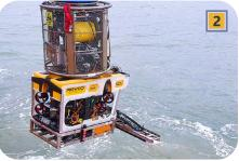
Work-Class ROV, enabling detailed surveys of areas of interest such as inspection of cable crossings, or archaeological surveys. Deployment with Pilot Assist / RPL following capability.
