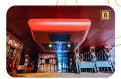
Hull mounted survey sensors enable high quality, repeatable MBES (2x R2sonic 2026) and SBP (1x Innomar Medium-100) data collection.
