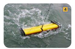
Equipped to deploy towed sensors such as SSS, ROTV or 2D-UHR.
