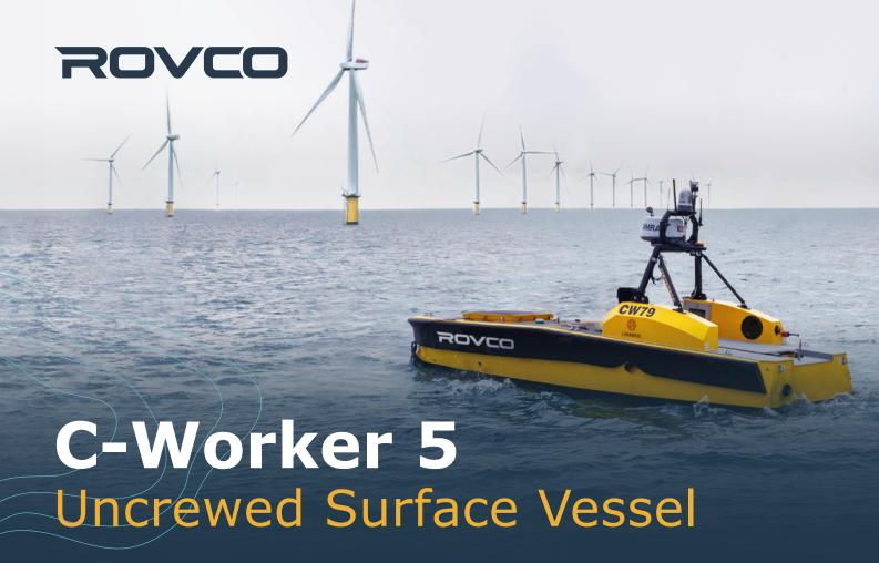
The C-Worker 5 is an autonomous vehicle designed to support hydrographic survey work and to increase survey coverage in limited timeframes. A proven offshore survey "force-multiplier", the vehicle will operate from the Glomar Supporter mothership, in supervised autonomy mode.
